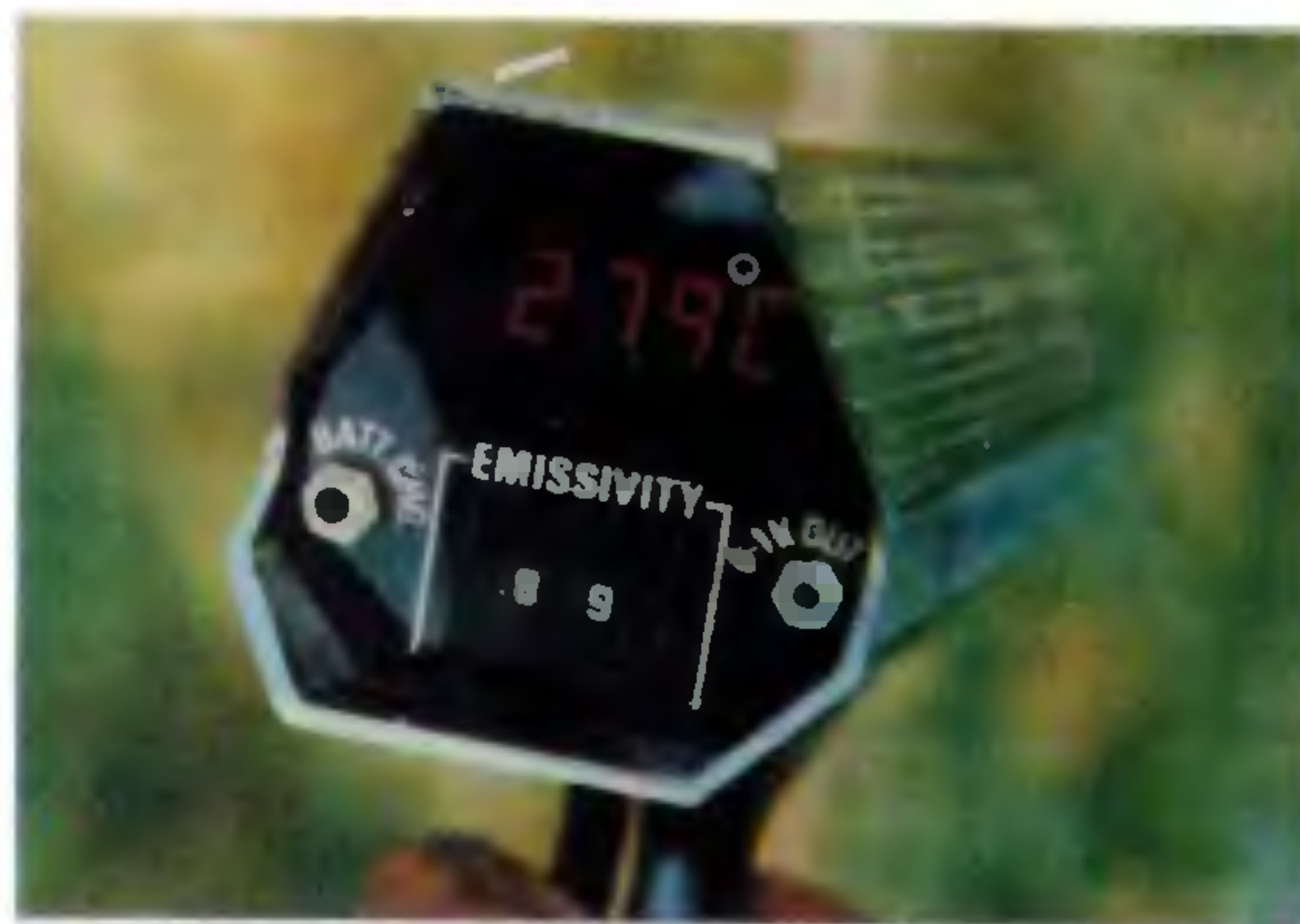
Figure 5. The infra-red gun measures canopy temperatures in the field. It also gives a measurement of crop canopy air temperature difference.
