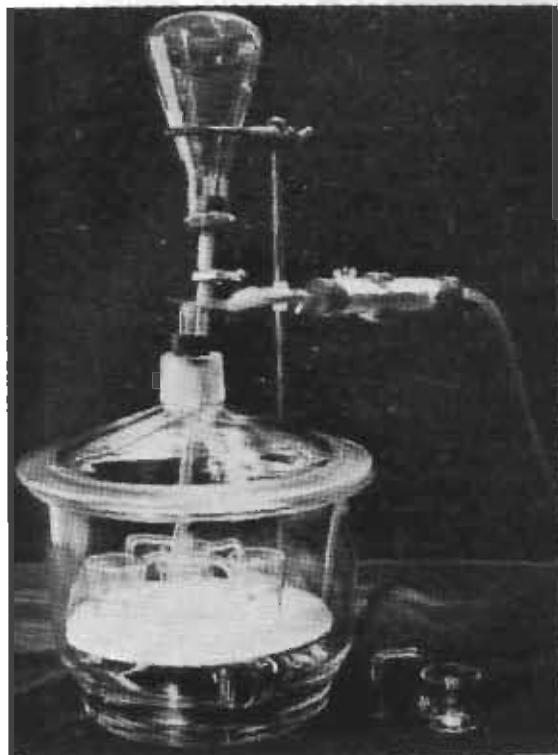
FIG. 3. Modified Plunkett chamber. Culture medium is sterilized in situ in the culture beakers. When cool, the level of liquid in the culture beakers is raised by attachment of reservoir at top, which contains sterile water. Sterile air is passed through the cotton-filled tube on right and is discharged below the supporting plate.
