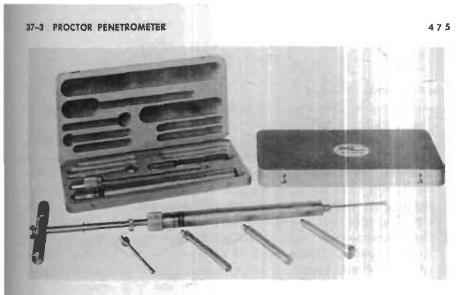
Fig. 37-2. Proctor penetrometer set.
