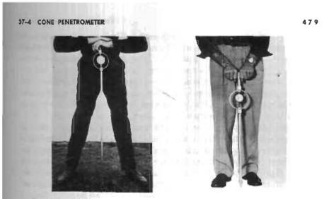
Fig. 37-4. Cone penetrometers (military model, left; commercial model, right).
