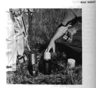
Fig. 30-1. Typical double-cylinder, hammer-driven core sampler for obtaining soil samples for bulk density.
