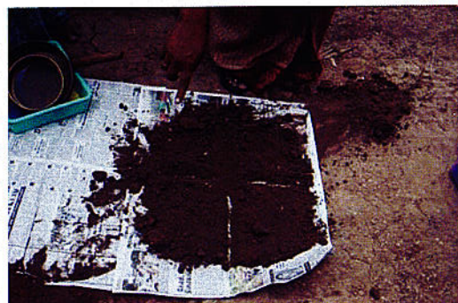
Fig. 3. Quartering method for sample size reduction
