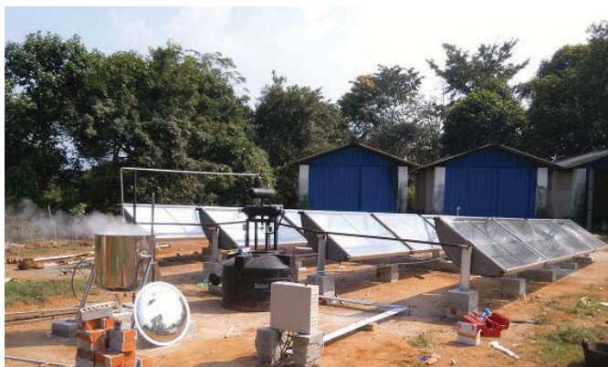
Turmeric being cooked by solar powered steam generator
