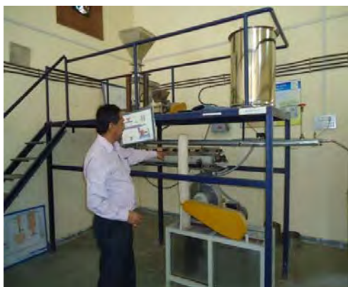
Fig 7. Cryogenic grinding facility for seed spices Fig 8. Processing facility for seed spice at Mehsana
