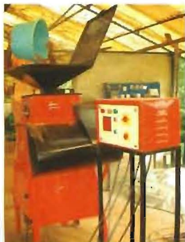
Fig 2. Machine for mixing and vending potting mixture
